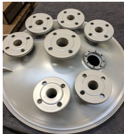
Tank top coated with Accotron BF
