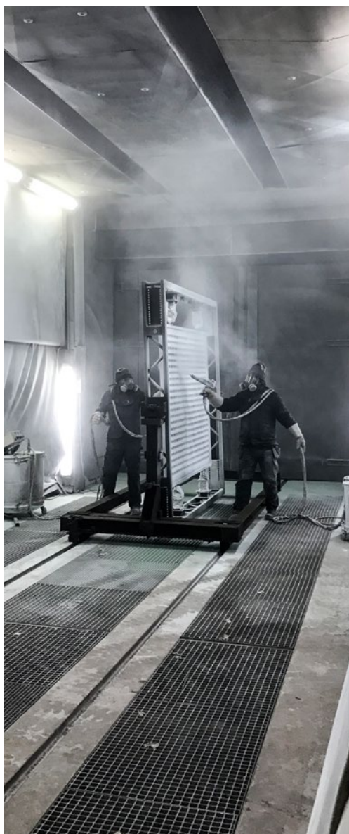
Accoat – coating with Accoshield powder
