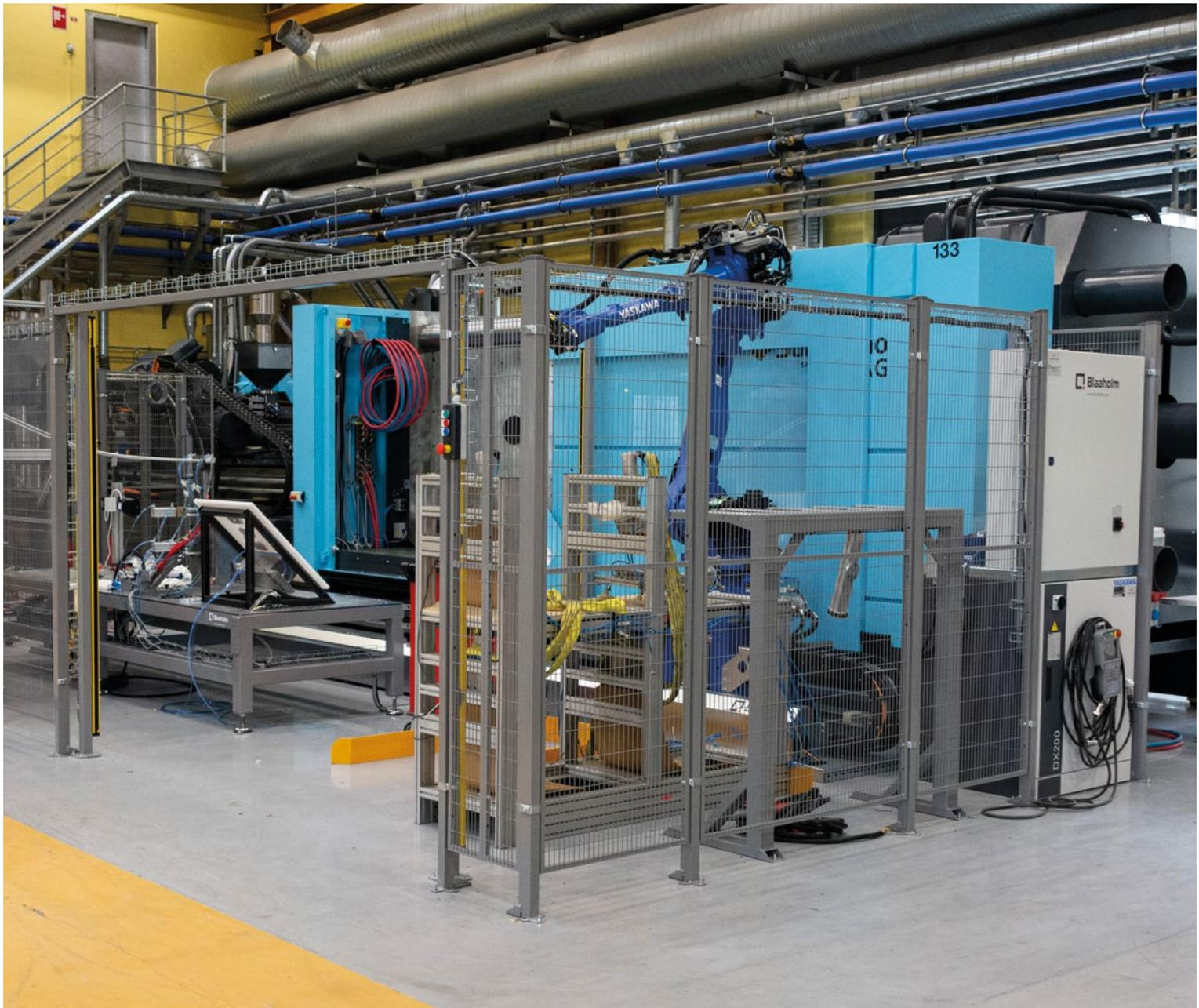
One of SP Moulding's new 1500T injection moulding machines.
