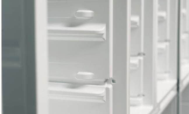
Vacuum formed inner box for refrigerators
